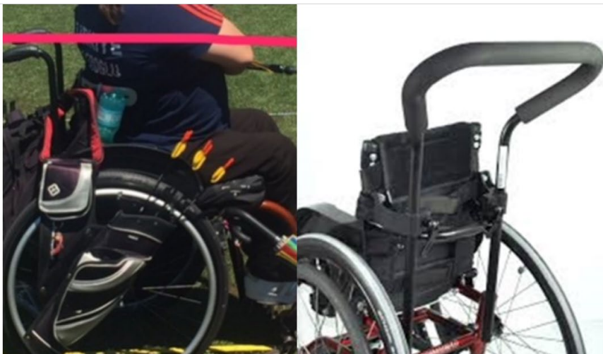
Image 3: Push Handles Not Attached to Wheelchair Back
